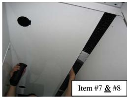
Slide the ceiling sections out of the way in order to access A/C hoses, wires, etc.
